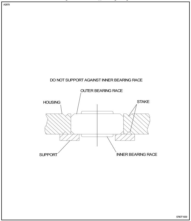
Figure 404: Sheet 1: Staking Tool - Typical
