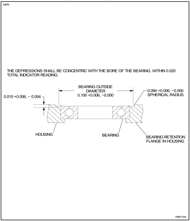
Figure 403 : Sheet 1 : Support During Staking
